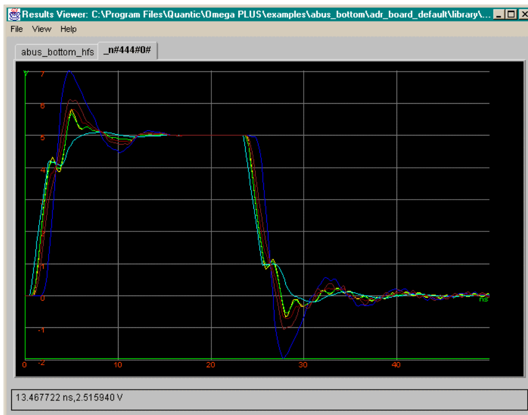
Figure 3. Voltage waveshapes at all pins on the dominant net.
